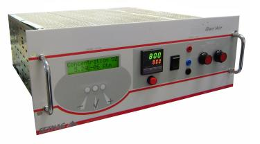
The GEN'AIR allows generating and measuring several different oxygen atmospheres. It's technology is based on the zirconia ionic conduction principle.
