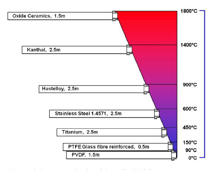
Maximum sample tube temperature is depending on the horizontal length inside this temperature zone
