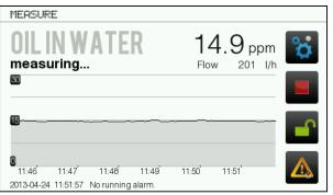
**Graphic interface** display of concentration & flow, easy setting, functional tests through touch screen.
